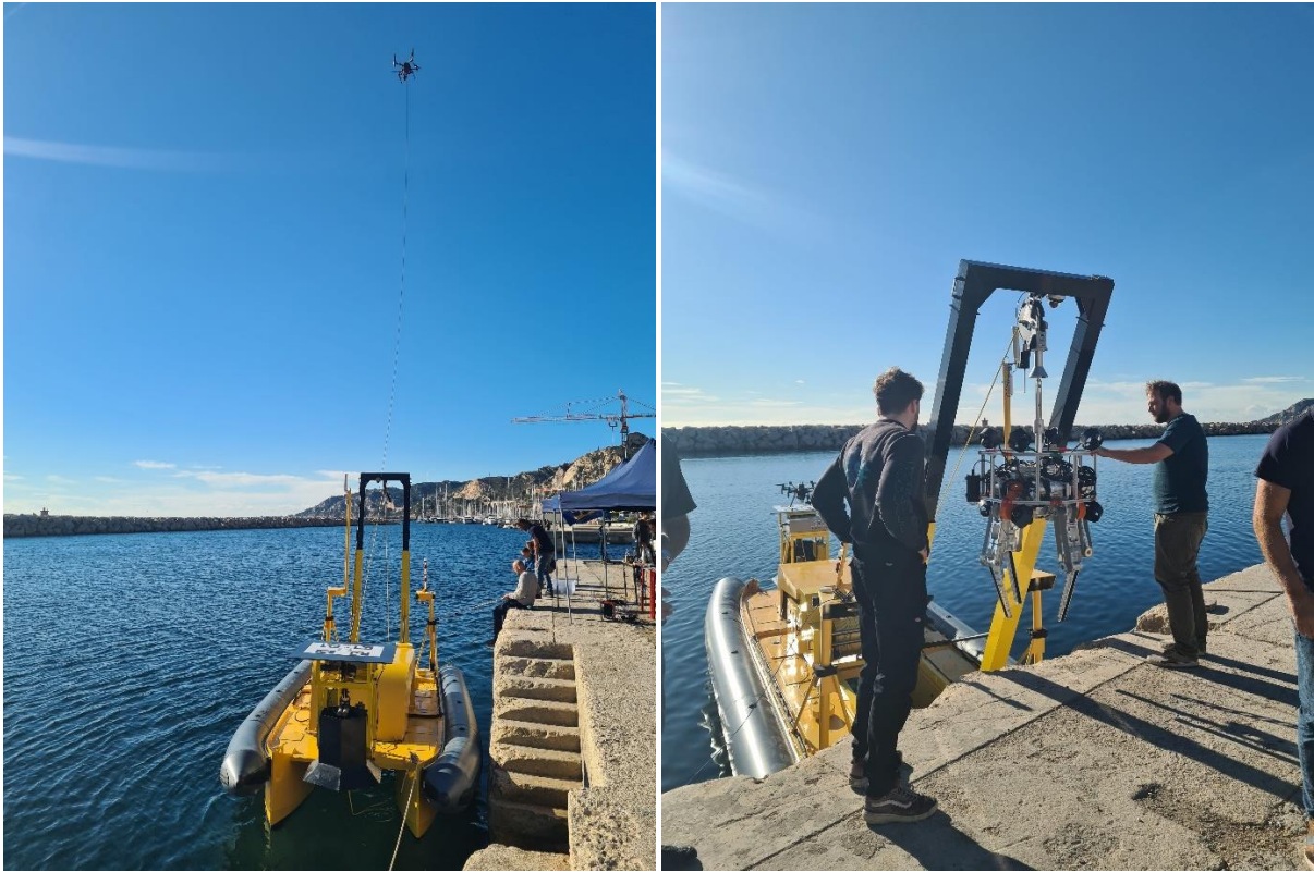
Figure 13: UAV tests above water and grapple connection to lifting frame.
