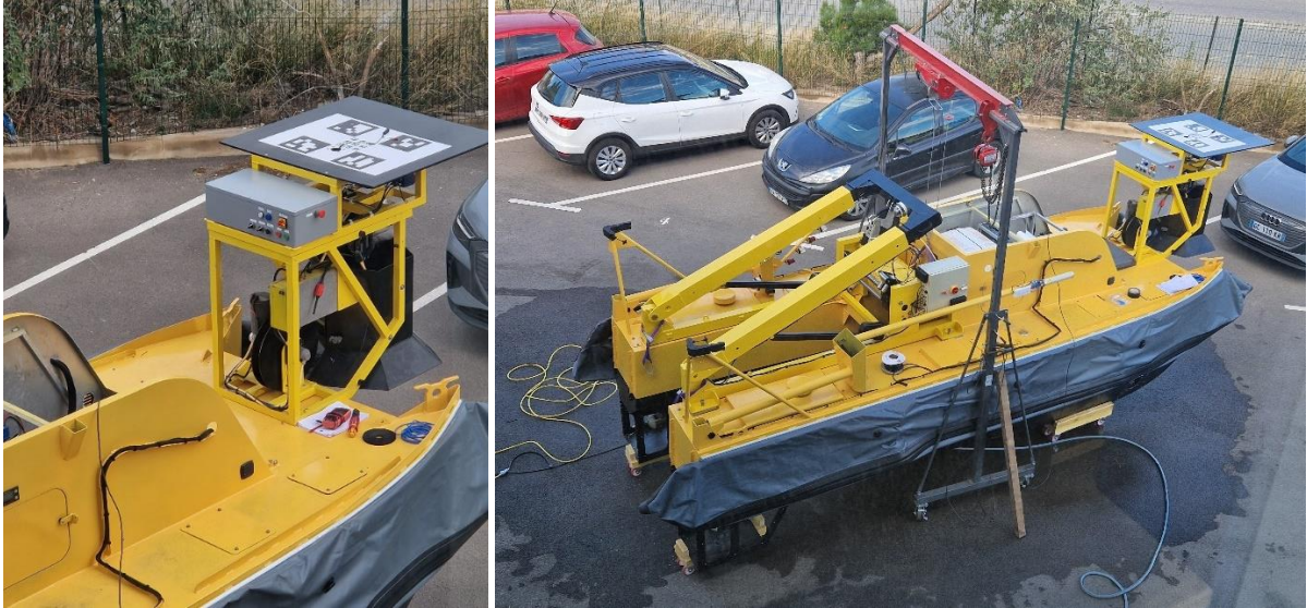
Figure 11: UAV platform & winch mounted on ROV LARS and grapple frame mounted on SeaCAT on Wednesday 18th
