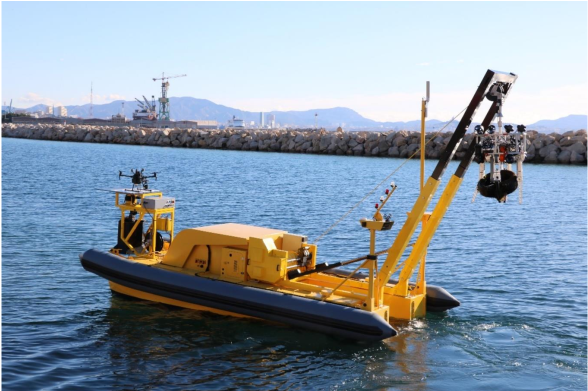
Figure 2: Overview of the SeaClear2.0 hardware system tested in Marseille.
