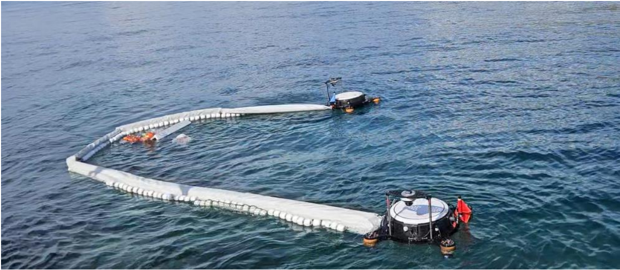
Figure 23: Testing of the upgraded collection net and the upgraded propulsion
