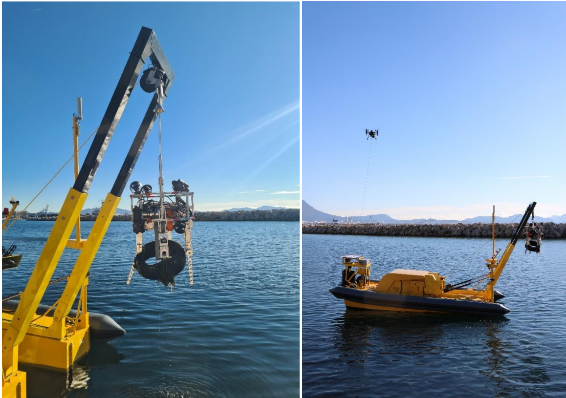
Figure 15: Tire lifted out of the water and last UAV flight from the SeaCAT in the channel
