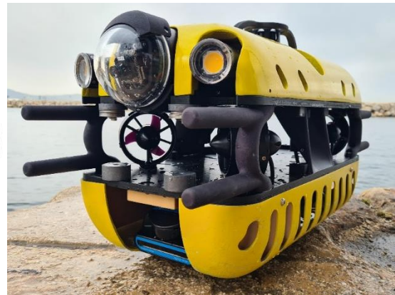
Figure 6: Blueprint Oculus M3000d mounted on Mini-Tortuga ROV
