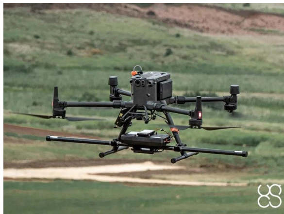
Figure 17: Example of magnetic sensor for UAV (SENSYS)
