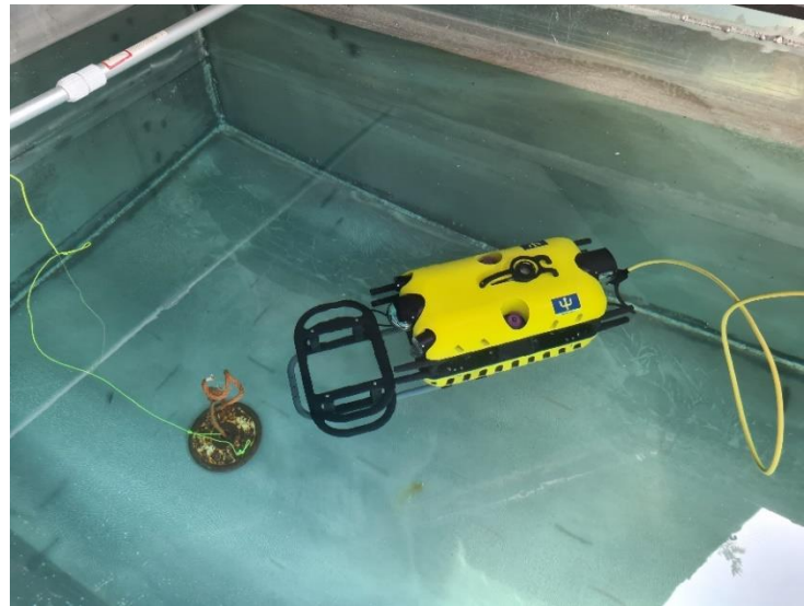
Figure 16: JW Fisher metal detector on Mini-Tortuga ROV, during preliminary tests
