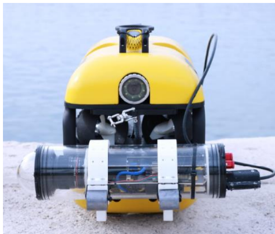
Figure 24: QCell multispectral camera on Mini-Tortuga ROV
