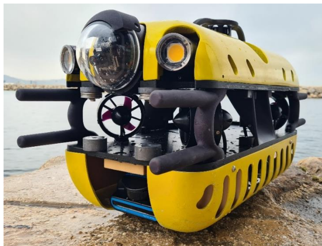
Figure 4: Subsea Tech inspection class ROV Mini-Tortuga
